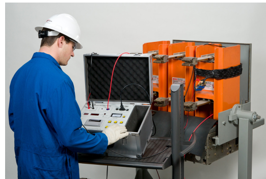
Figure 9. Flexible magnetic field coil applied to an entire pole.
