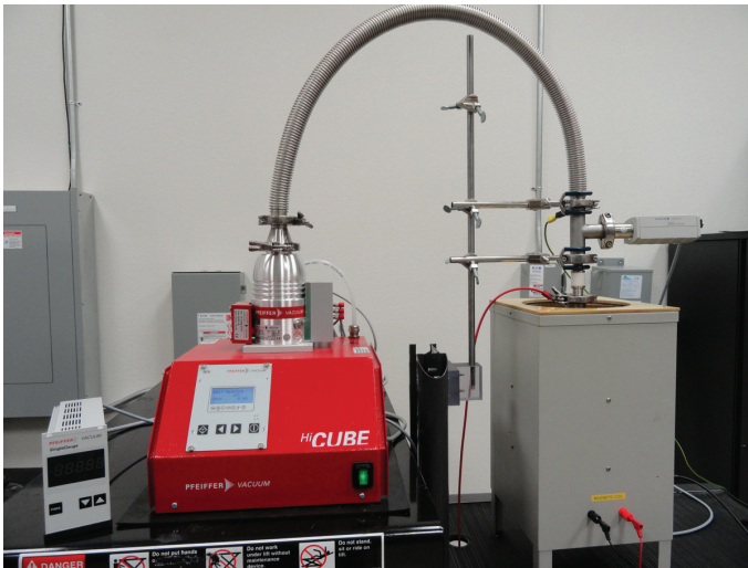
Figure 10. Test setup for developing vacuum versus current data.
