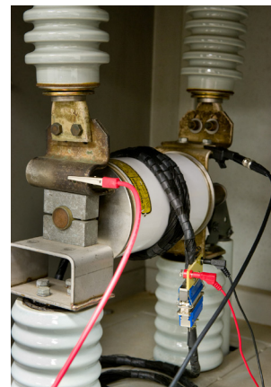
Figure 8. A newly designed flexible magnetic field coil for field testing.
