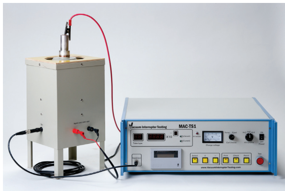
Figure 7. Stand mounted coil for application of uniform magnetic field.
